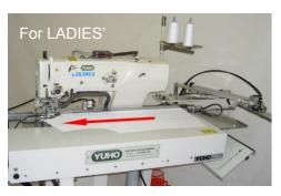
Just put front body panels on the table. Operators do not need to pay attention to the positioning of left or right strictly. This feature enables higher productivity.
