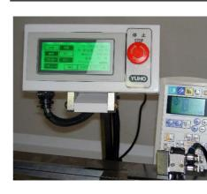
Various parameters such as distance from the upper end to the top button, button intervals, # of buttons, bobbin counter, pattern # etc. are displayed at once on the touch panel, allowing users to change settings with
