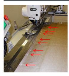
Up to 20 patterns of button hole intervals can be stored as equal intervals. In the case of unequal intervals, users can differentiate each interval as they like by inputting each distance one by one on the touch panel. Up to 20 patterns can be stored as unequal intervals.
