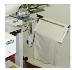
Stacker mechanism on the right side of machine piles up front body panels of both MEN and LADIES. (MEN: top is right, LADIES: top is left) Thanks to its stacker turn-over shaft, materials are piled up tidily.
