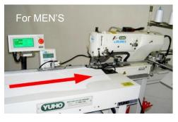
U-2604-BH comes with the Direct-Drive Motor type machine head (max. 4200 rpm sewing speed). Its electronic thread tension control system
