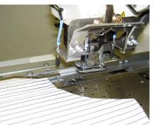
This machine detects the upper edge of front body panel using photoelectric sensor and feeds it with vacuum plate without clamp. Consequently, it has a flexibility to change the position of top button hole which
