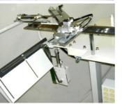
The stacker mechanism on the left side of the machine piles up front body panels of both MEN'S and LADIES'. (MEN'S: top is on the left, LADIES': top is on the right) Thanks to its stacker turnover shaft, materials are
