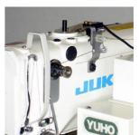
T.B.D. detects the thread breakage and stops the machine immediately. Operator can choose to step back or step forward before restarting, reducing waste of time and extra work.
