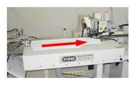
This machine detects the upper edge of the front body panel using a photoelectric sensor and feeds it with a vacuum plate instead of
