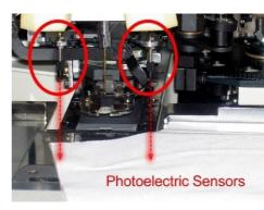
Just put the front body panels on the table. Operators do not need to pay strict attention to the positioning of left or right. This feature enables high productivity. 2 x photoelectric
