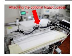
With the optional Robot Loader, unmanned operation of the entire production process including loading, button sewing, and stacking is possible. Since the Robot Loader synchronizes with the
