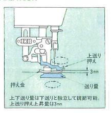
Reasonable Top-feeding synchronized with Drop-feeding, Partial-gathering equipment (**PF-6**) various Attachments ---support the Beginner's operatio nsimply.
