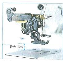
With high Presser-foot up, internalized Top-feeding, fabric Loading, Handling is allowed easily. Stitching-pitch Dial is very variable and handiness to the Operators.
