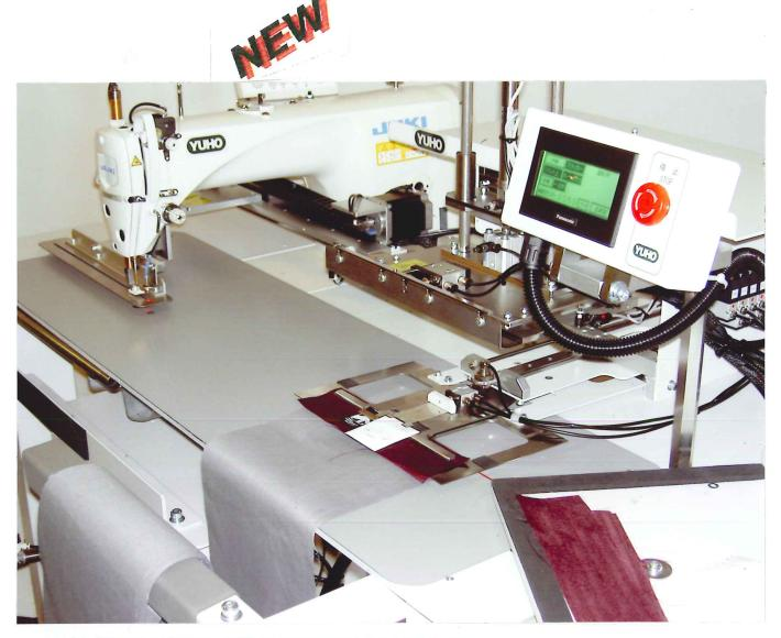
**U-3203-E/LW NEW POCKET FACING SEAMER**---faces a Patch to the Side-Pocket automatically in **"L"** pattern---with "Consistent Seaming"
