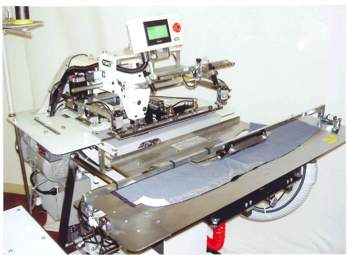
NEWLY DESIGNED NEW NC BREAST DART SEAMER U-3207-E/300 & /LM TYPE WITH NUMERICAL PROGRAMMABLE BY "LED" TOUCH PANEL IS NOW APPLICABLE TO VARIOUS PATTERN SIZE SETTING FLEXIBLELY AS DESIGNED !!
