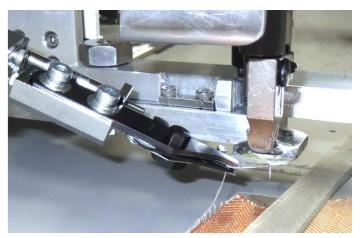
In order to avoid troubles at the beginning of each seam line, the U-3707 pulls thread using the Thread Clamper. Right after cutting the thread by knife at the end of the previous seam line, the Thread Clamper catches the thread, and releases it as soon as the needle moves. Since this procedure automatically takes place repeatedly at every single seam line, you are completely free from stitching troubles.
