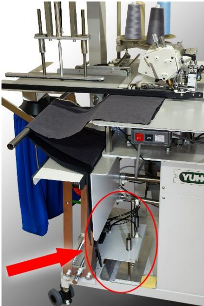
Elevator type lower table removed and stored on the machine
