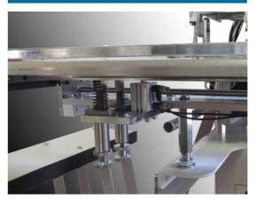
The height and horizontal level of the top of the fabric setting table are adjustable instantly and precisely. This feature is advantageous for handling various materials with different thicknesses at the stage of setting materials between the loading plate and fabric setting table.
