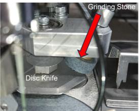
The disc knife is made of high-speed steel, making it highly durable, easy to remove and polish, and, as standard, equipped with a grinding stone, allowing it to maintain its sharpness at all times.
