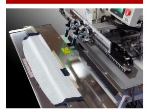
When sewing darts for semi-custom-made jackets, each front panel has a breast dart of a different size and shape. U-4001 can manage variety of dart lengths one by one by simply aligning the projected cross marks of marking lights with the marks on each material (marked by eyelet or marking pen), indicating the dart's Halfway Point and the End Point. (Note: The depth of the darts must be set separately.) Since this machine sets the materials based on the pocket opening of the waist
