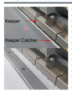
U-4002's keeper is made out of a single piece of a long metal plate; thus, the keeper's teeth are always kept aligned. Besides, thanks to the combination of keeper and keeper the U-4002 catcher. securely grabs various of varying fabrics thicknesses. A keeper catcher also helps prevent the keeper from making scratches with its teeth on the table's surface.
