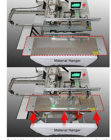
A material hanger is provided just in front of the vacuum suction plate, allowing operators to load fabrics more quickly. The vacuum plate moves toward the sewing head, allowing sufficient space for the operators' hands when putting the bunch of materials.
