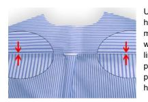
Using the yoke piece with horizontally striped materials requires a line of welt seaming stitches and a line of flipovers on the yoke piece and must be paralleled with the horizontal stripes.
