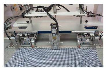
Two sets of keeper units (Left & Right), a center keeper unit, and vacuum suction functionality on the table surface are available for perfectly loading materials. Besides, the newly equipped needle-type keeper unit supports holding pleats (where the materials are layered) and prevents slippage of materials.
