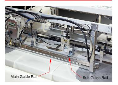
Due to the double chain stitch sewing head, the U-4007 guarantees high-quality seam lines with stretchability but without puckering. Furthermore, three-layered materials are held down securely and conveyed by two guide rails (main and sub) to keep the seaming area under the needle in perfect condition. This mechanism is the key to securing the highest quality of sewing.
