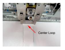
to insert the center loop along the loop-attaching device, and then the machine sews the center loop together with yoke pieces and back panel all at once. The machine accepts a center loop with a minimum of 30 mm to a maximum length of 40 mm, and operators can easily optimize machine settings depending on size just by turning a knob.
