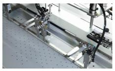
The mechanisms for folding devices (Left & Right) allow them to move symmetrically, so operators only need to touch one side and can set
