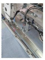
panel, and the main guide rail, synced with the sub-guide rail, conveys them to the needle. This mechanism contributes to perfect welt seaming without puckering while reducing cycle time.
