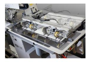
The auto feeder section employs 4 x adhesive tapes to guarantee secure and stable picking of materials one by one. Just 0.2 mm of the adhesive surface is automatically supplied and rolled up whenever it picks each material up. The operator can set the locations of picking up/releasing precisely and instantly by inputting on the touchscreen. Each feeder unit uses 2 x adhesive tapes, and the
