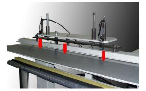
After the double-fold process, both left and right sides of the front placket are steadily held down by the guide rail and transported under the needle for stitching, then transported again under to the heat pressing area. The quide rail releases the material while the vacuum suction keeps the material right under the heat pressing element, and it goes down and presses the material.
