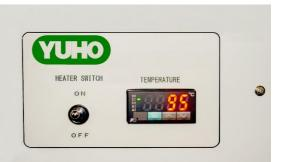
Heat pressing temperature, as well as the duration, can be set in detail individually.
