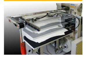
The lift-type tray of the auto-loading unit supports the materials with a maximum size of 750 mm(W) x 300 mm(D), and the loadable amount of content up to a height of 180 mm. The lift always detects the height of the stack, and automatically lift it so that the top of the material always keeps the same height. The auto loading unit automatically stops operation when the tray is empty.
