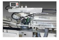
pedal is pressed, making it easy to check and adjust each device and confirm the sequence order. Also, when performing maintenance on the sewing head, it is possible to easily tilt and tilt back the sewing head to its original position.
