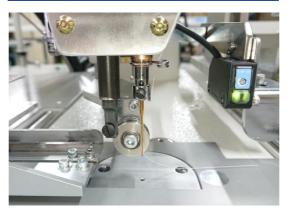
The bobbin thread must come to the surface side when making the shirt front placket using the conventional binder/hemmer. U-4202 allows needle thread to appear on the surface side, securing a beautiful stitch seam line.
