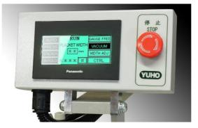
Besides the placket width, the operator can set or change various functions and parameters of devices instantly just by touching the LCD. This machine's Intuitive touchscreen system allows hassle-free operation, even for the lessexperienced beginner workers.
