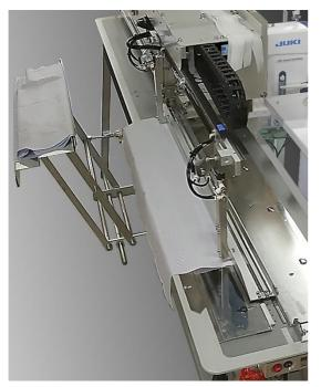
The materials are held by a powerful vacuum suction installed on the surface of the work table of U-4202 and are steadily hemmed by an onboard double-fold device. Immediately after, the materials are conveyed to the needle, securely held by a guide rail, and stitched straightaway.
