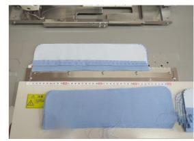
Place two pieces of material layered on the table with the vacuum suction activated. Next, when folding a part of the overlaid piece, step on the pedal to increase the vacuum suction and the vacuum will keep the folded condition, so make sure to insert the mountain folded part under the claw of the guide ruler. Pull it toward operator and align the edge of the mountain fold precisely with the horizontal edge of the guide ruler, and also align it perfectly with the left edge of the guide ruler.
