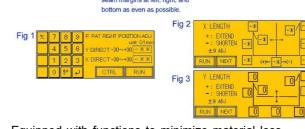
Equipped with functions to minimize material loss and idle time by automatically stopping the operation when thread breakage occurs or when the amount of bobbin thread remaining is low. These settings and adjustments can be easily made on the touchscreen.
