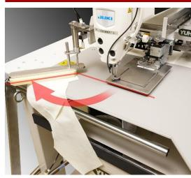
U-4304 automatically sews coin pockets onto pocket bag material and rotates it 90 to 120 degrees. Its stacker device with the turn-over bar neatly aligns and stacks the materials. This stacker with the swing pat allows significant overlap between the material setting/folding process and the sewing and stacking processes, tremendously contributing to higher productivity and efficiency.
