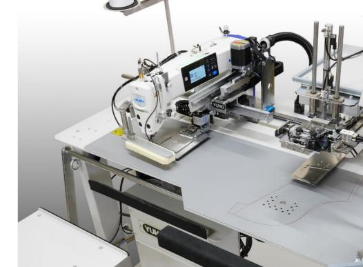
YUHO's Coin Pocket Setter, which boasts the same superior functionality as YUHO's acclaimed Pocket Setter U-4203 and executes high-quality coin pocket attaching to pants pocket bags, is now available with the latest lockstitch digital sewing head onboard.
