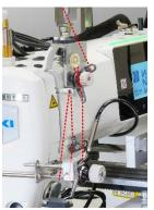
Production loss time and material loss are kept to a minimum by quickly detecting thread breakage and automatically stopping operation.
