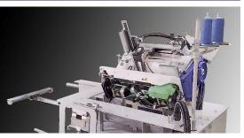
The mechanical structure is carefully designed to eliminate the need for readjustment when tilting and returning the sewing head, reducing maintenance burdens. The LCD touchscreen also includes a variety of maintenance menus to cope with just in case any trouble should occur, such as test stitching of the sewing head independently and correction of delicate settings of each device together with the functionality of step-by-step playback of preprogrammed sequence.
