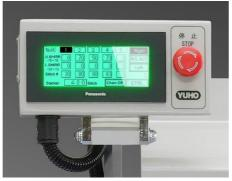
"Continuous left," "Continuous right," and "Alternate left/right." When "Alternate left/right" is selected, the left and right operations switch automatically and instantly. In addition, up to 40 sewing patterns can be stored and recalled with a single touch on the LCD touchscreen.
