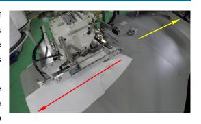
guide, the right end of the material is temporarily held by the Fabrick-End Keeper device and transported to the stacker to eliminate misalignment at the end of materials and ensuring the trimming of chain-off threads.
